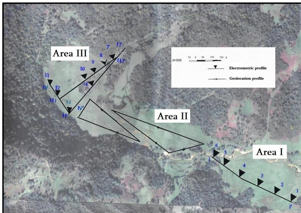
The cross sections made by vertical electronic sensing and radiolocation methods combine each other; the results obtained are in good harmony with each other and uniquely depict the real karst and geological environment.
