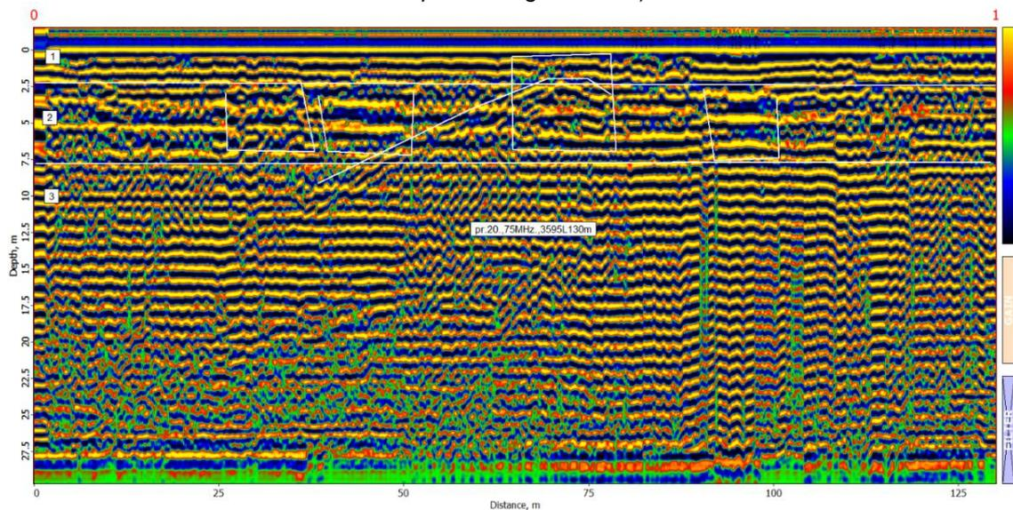
According to the texture of the synphasing axes, three georadiolocation layers were distinguished on the Profile № 33 (Fig.12): the first layer – with a capacity of about 2 m, the second layer – 7.5 m and the third layer extends below 7.5 m. The first layer is more or less uniform and partially disintegrated. The second layer contains the radioimages of hydrated water-permeable areas. The third layer does not contain significant cavities; the moistened area is marked below 20 meters.
