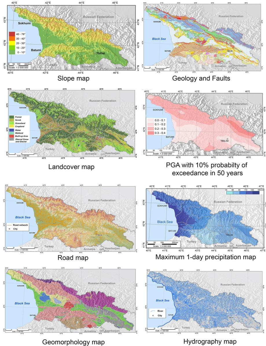
**Fig. 7** Factor maps used in the landslide susceptibility assessment. For the geological and geomorphological maps, no legends can be shown as there are too many units. Higher-resolution maps with complete legends can be downloaded from: [http://drm.cenn.org/paper\\_atlas/RA-part-2.pdf](http://drm.cenn.org/paper_atlas/RA-part-2.pdf)
